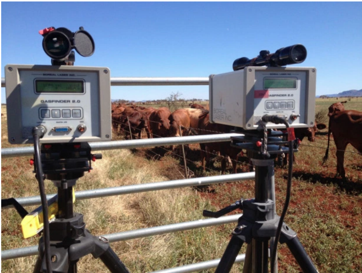
Rob Kinley An open path laser measures methane in the field.
